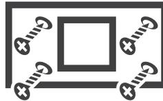
Use sheet metal screws provided to secure the UV air sanitizer
